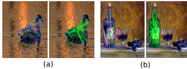
Fig. 4. Left plot in panels (a) and (b) shows standard Hough voting which assumes mutual independence between features. Right plot in panels (a) and (b) shows the voting after joint optimization of correspondences, groups, and votes.
