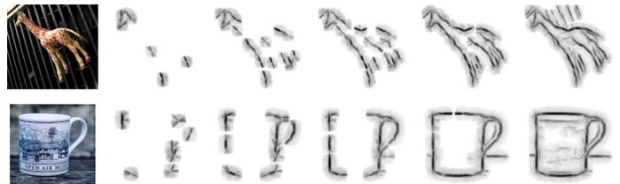
Figure 2: Shape information is concentrated at points of high curvature. Oriented bar features are ordered and rendered by contour strength and curvature using 10, 30, 50, 100 and 200 features.
