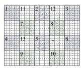
Fig. 4. Scheme of blocks and update schedule used for the Block-ICM algorithm. In every odd sweep, square blocks ( $6 \times 6$  sites in the figure) are visited following the pattern indicated by the numbering. The even sweeps are performed in the same way but shifted by half a block (dashed squares).
