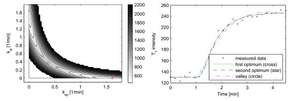
Fig. 3. Left: Projected NLS objective  $f(k_{\rm el}, k_{\rm ep}) = \min_{S_0, A, t_0} J(\boldsymbol{\theta})$  s.t.  $k_{\rm ep} > 0$  and  $k_{\rm el} > 0$  for another example from the prostate data set. Right: The corresponding data fits reveal that the two optima (cross and star) yield the same model curve which reflects that the employed model is not identifiable.
