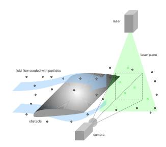
Fig. 1. Particle Image Velocimetry (PIV) experimental setup: The flow of a fluid behind an obstacle shall be examined. To this end, it is seeded with small particles. A laser projects a thin plane into the region of interest and illuminates the particles therein. Fluid motion can be measured by analysing the image sequence recorded by a camera system.
