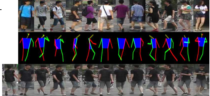
Figure 6: Appearance transfer on Market-1501. Appearance is provided by image on bottom left. \hat{y} (middle) is automatically extracted from image at the top and transferred to bottom.
