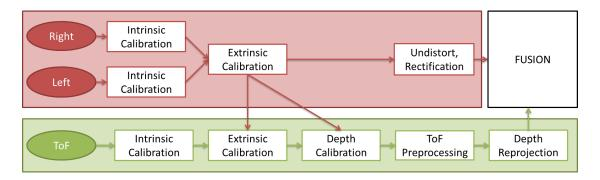
Figure 2: Basic Fusion Pipeline
