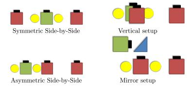
Figure 3: Different possible camera setups. Green: ToF Camera, Red: RGB Camera, Yellow: ToF Lights
