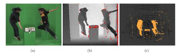
Figure 5: Ruhl et al. – input data example: approximate depth data from multiple unsynchronized Kinects to be used as uncertain prior to image correspondence estimation. (a) HD camera image, (b) VGA depth map (invalid depth data marked in red), (c) depth points projected into world space.
