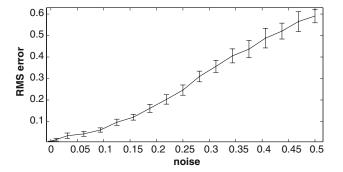
Fig. 14 RMS velocity error (in pixels) when adding different amounts of Gaussian noise (zero mean and variance up to 50%.)
