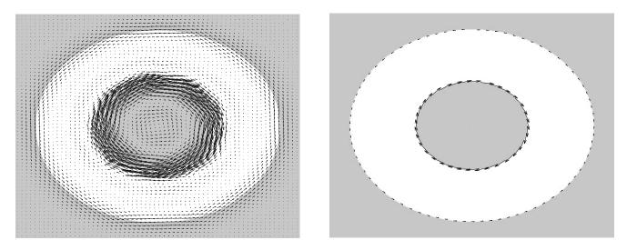
**Fig. 11** Reconstructed body force. *Left*: Penalization everywhere (force scaled by 10,000). *Right*: No penalization on interfaces (force scaled by 100). The frictional forces at the cylinder interfaces are extracted correctly
