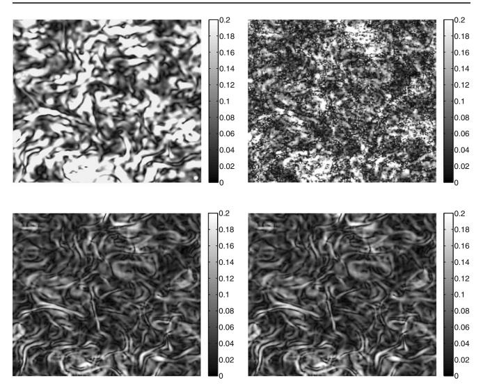
**Fig. 15** *Top left:* Multi-pass cross-correlation (DaVis), av. err. = 0.1420 pixel. *Top right:* Horn and Schunck, av. err. = 0.0821 pixel. *Bottom left:* 2nd order regularization, av. err. = 0.0525 pixel. *Bottom right:* Optical Stokes flow computation, av. err. = 0.0484 pixel
