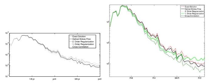
Fig. 17 Energy of the vorticity (for frequencies between 0 and  $\Pi/2$ ) of the different algorithms (logarithmic plot). Energy spectrum of optical Stokes flow estimate is closest to the true solution, while cross-correlation underestimates higher frequencies
