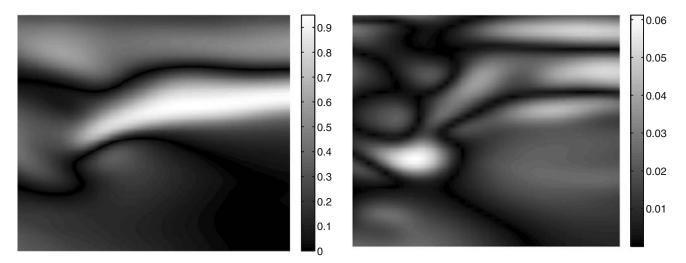
Fig. 21 Out-of-plane velocity (*left*) leads to divergence of the 2D projection (*right*). We have to use the modified optical Stokes flow approach to reliably reconstruct the target velocity field
