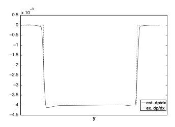
Fig. 7 Profile of the averaged pressure derivative in flow direction. Note that the linear pressure decrease in flow direction  $(-4 \times 10^{-3})$  inside the pipe) is recovered extremely accurately
