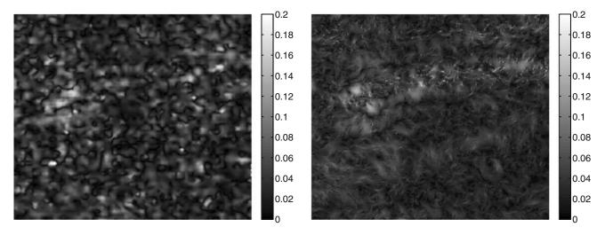
**Fig. 20** Left: RMS velocity error of cross-correlation approach (smallest window size  $16 \times 16$ , 50% overlap, mean RMS = 0.0331 pixel). Right: RMS velocity error of modified optical Stokes flow ( $\mu = 1$ ,  $\alpha = 100$ ,  $\beta = 200$ , mean RMS = 0.0212 pixel)
