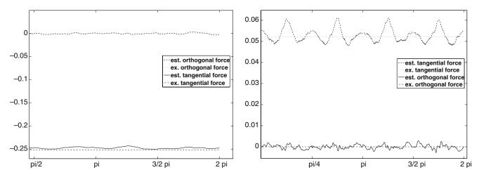
Fig. 12 Optical Stokes flow is able to compute the forces that act on the cylinder interfaces. *Left*: Tangential and orthogonal forces at the inner cylinder boundary. *Right*: Tangential and orthogonal forces at the outer cylinder boundary
