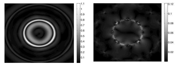
**Fig. 13** Left: RMS velocity error (av. 0.110 pixel) when penalizing the body force everywhere. Right: RMS velocity error (av. 0.0079 pixel) when no penalization on the cylinder boundaries is performed
