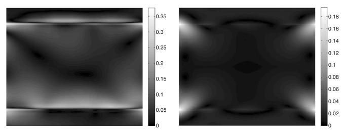
Fig. 6 Left: If we penalize **f** everywhere, the mean RMS error is 0.0734 pixels. Right: By specifying the solid–liquid interfaces, the RMS error decreases to 0.0212 pixels
