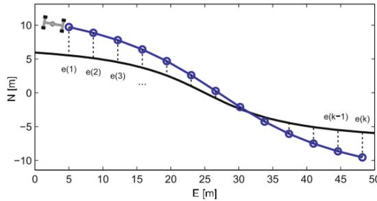
The deviation can be calculated by a function  $J$  that sums up the squared errors over a given time interval. These can represent the past and the predicted future.
