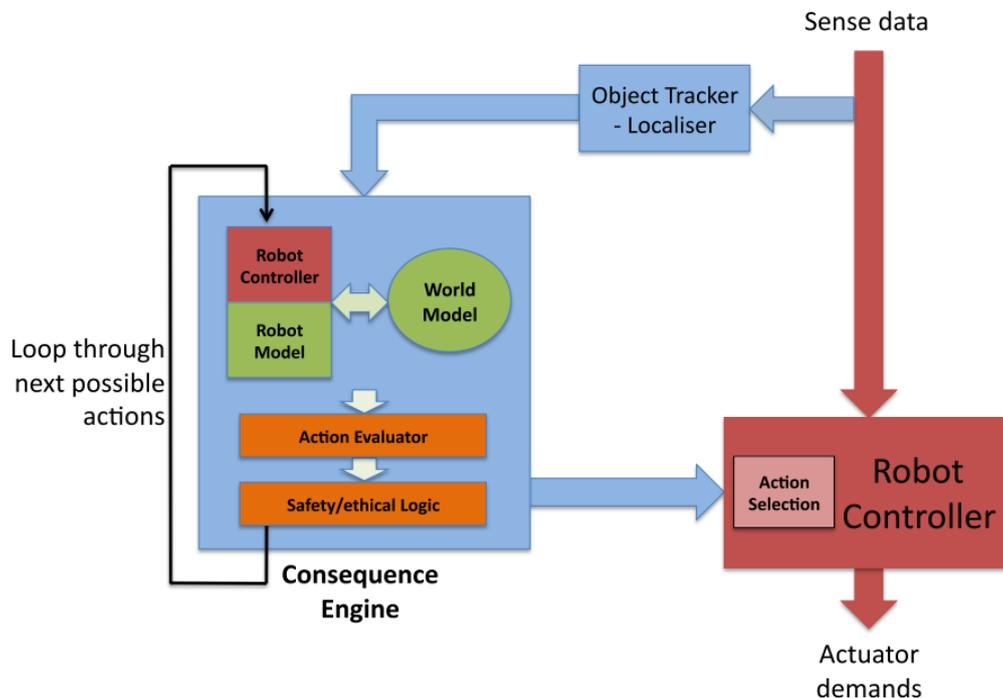
Figure 4.1: Architecture of the consequence engine by [3]
