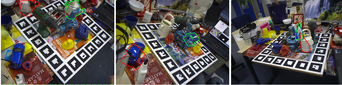
Figure 5. Qualitative results of our method on the ‘‘Occluded Object Dataset’’ [3]. Results of our method are depicted as green silhouettes, the ground truth pose is shown as a blue silhouette and results of the method by Krull et al. [19] are shown as red silhouettes. Note, since these results shows correct poses of our method the green silhouette is on top of the blue one.
