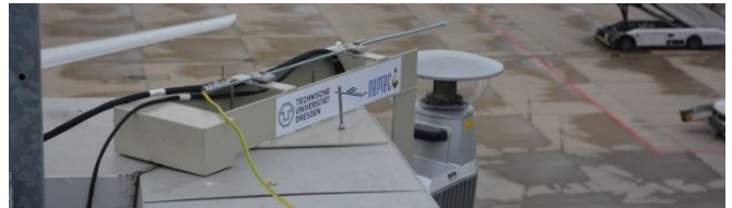
Figure 8. LiDAR sensor mounted at Dresden airport
