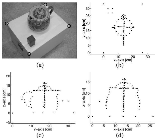
**Figure 3. Original view (a), top (b), side (c) and front (d) view of the reconstruction. The dots represent the reconstructed model points.**
