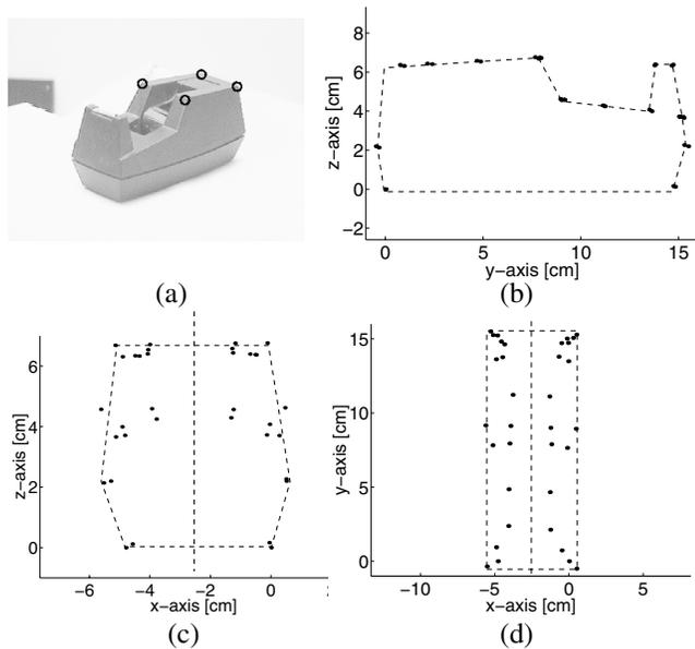
**Figure 2. Original view (a), side (b), top (c) and front (d) view of the reconstruction. The dots represent the reconstructed model points and the dashed lines display the contour and the symmetry axis of the model.**
