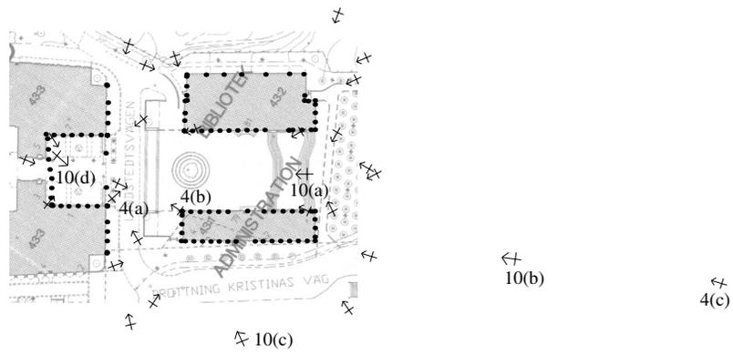
Figure 8. Top view of the reconstruction of the campus with 114 model points (dots) and 27 cameras (arrows). A map of the campus is superimposed. The labeled cameras correspond to images in the respective figures.
