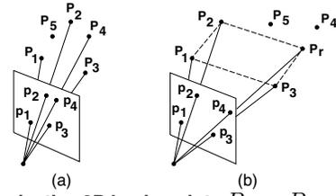
Figure 1. Projective 3D basis points  $P_1 \dots P_5$  and image basis points  $p_1 \dots p_4$  for general configurations (a) and reference plane configurations (b).
