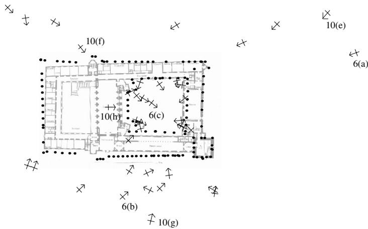
Figure 9. Top view of the reconstruction of the City Hall with 129 model points (dots) and 35 cameras (arrows). A map of the City Hall is superimposed. The labeled cameras correspond to images in the respective figures.
