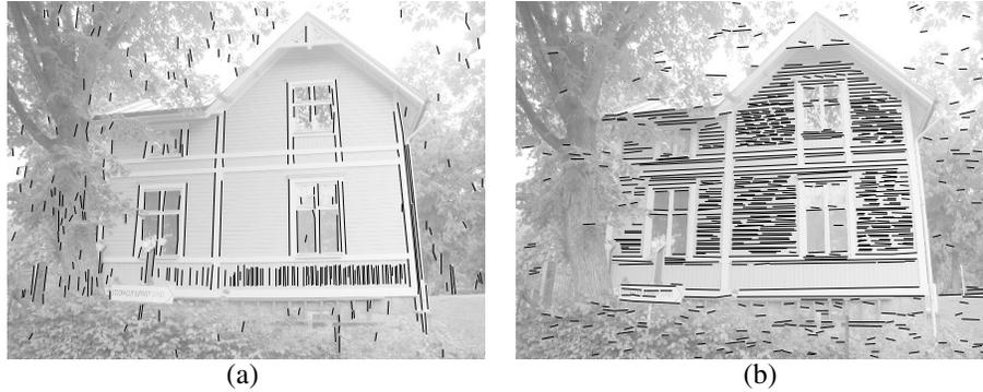
**Figure 8.4.** The 1174 line segments in fig. 8.1(b) were classified into two dominant directions. The first direction (a) is supported by 308 line segments. The second direction (b) by 643 line segments. The remaining 223 line segments were classified as outliers.
