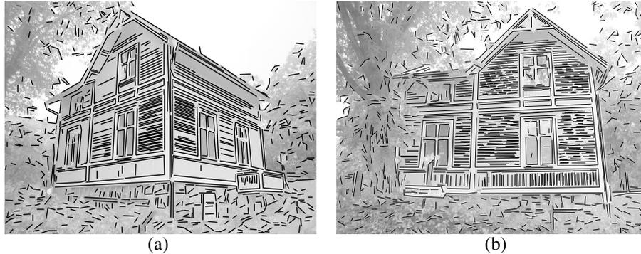
**Figure 8.1.** Two images of the house sequence. In (a) 846 and in (b) 1174 line segments were detected automatically.
