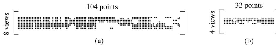
**Figure 6.13.** The visibility matrix of the teapot (a) and the tape holder (b). If the  $j$ th point is visible in the  $i$ th view, the corresponding element  $V(i, j)$  is set (a black square).
