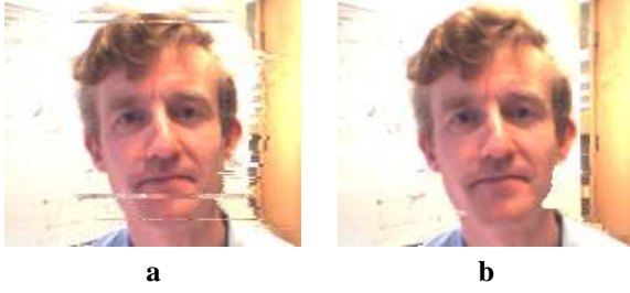
Fig. 28. Example of gaze correction. (a) Cyclopean image synthesized via the algorithm in [COL93]. This image is identical to that in fig. 3b and is repeated here for clarity. The input left and right images are shown in fig. 3a,c, respectively. (b) The cyclopean, gaze-corrected view generated by our algorithm. The gaze has been corrected while eliminating the artefacts of (a).
