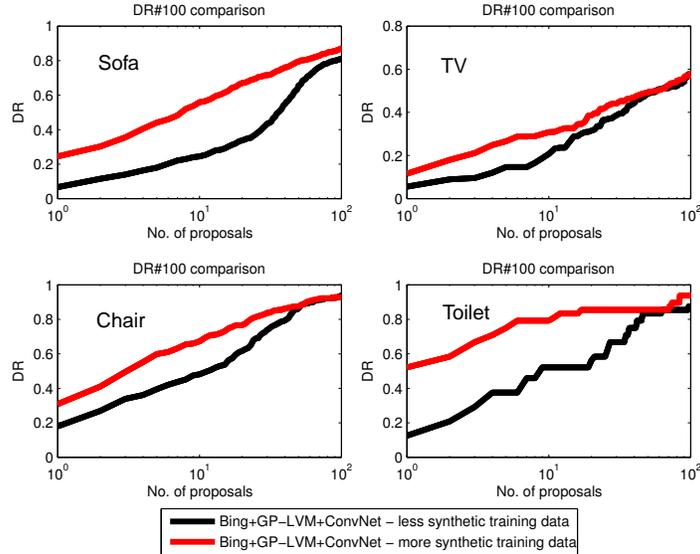
**Fig. 5.** Logarithmic plot measuring the DR#100 (50% Intersection-over-union) accuracy when we double the amount of synthetic data (i.e. sofa: 43200 (red), 21600 (black); TV: 50400 (red), 25200 (black); chair: 74800 (red), 37400 (black); toilet: 28800 (red), 14400 (black)). The extra data leads to much higher accuracy when using fewer proposals. As the number of proposals increases the extra training points do not help much, as the BING discrimination ability saturates.
