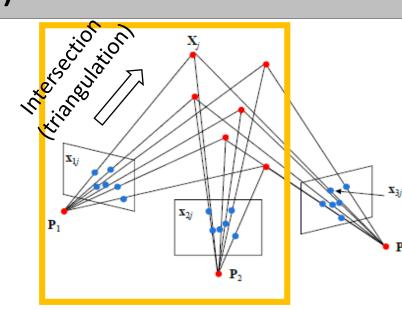
2) Eliminate λ by taking ratios. This gives 2x2 linear-independent equations for 4 unknowns: X = (X<sub>1</sub>, X<sub>2</sub>, X<sub>3</sub>, X<sub>4</sub>), and we want: ||X|| = 1. (remember X is a homogenous 4D vector, hence scale has to be fixed)
