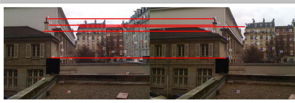
$$\begin{array}{l} \underline{Algorithm:}\\ 1) \mbox{ Take } m \geq 4 \mbox{ point matches } (x,x')\\ 2) \mbox{ Assemble } A \mbox{ with } A {m h} \ = \ 0\\ 3) \mbox{ compute } {m h}^* = argmin_{{m h}} \|A{m h}\| \mbox{ subject to } \|{m h}\| = 1,\\ \mbox{ use SVD to do this.} \end{array}$$
